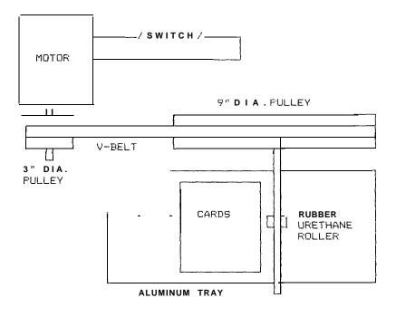
Figure 2: A schematic of the card sorter unit
