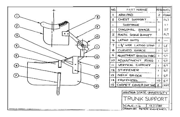
system. The second component consists of an adjustable linkage and the chest support. The adjustable linkage allows adjustment to fit a range of rider sizes. The chest support, which is made of polypropylene plastic, is attached to the adjustable linkage. For comfort it has covered foam padding under the arm area. Once the device has been adjusted to the individual, the chest support can be easily and quickly detached from the plastic saddle blanket, allowing for easy mounting and dismounting.
