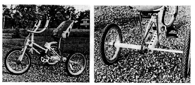
To facilitate getting the child on and off the bike, a parking brake was added to the front wheel. This brake is actuated by a simple lever, similar to a wheelchair brake.
