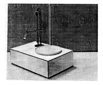
Both these motions are controlled by the joystick. A lazy susan device allows the plate to rotate. The plate's rotation is controlled by pushing the fire button on the joystick. The power to the entire unit is supplied by the battery on her wheelchair.
