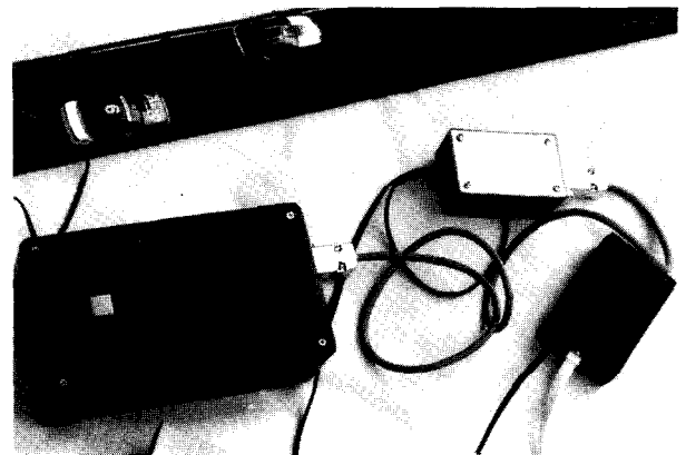
Fig. 11.7. The Myoelectric Muscle Car showing System Box with Turbo Button and Indicator Lights, the MMA, and an Interface Box.
