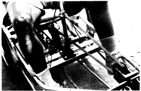
Fig. 14.3. Detail of T-bar, Strap, Cam, and 3-Speed Hub.
