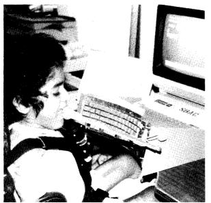
Fig. 14.5. Greg With New Mouth Probe and Keyboard. Note Probe Holder Attached to Keyboard for Easy Accessibility.
