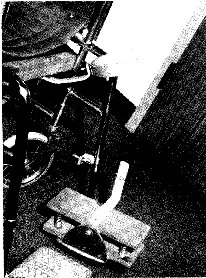
Fig. 17.7. Control Device for a Power Wheelchair.
