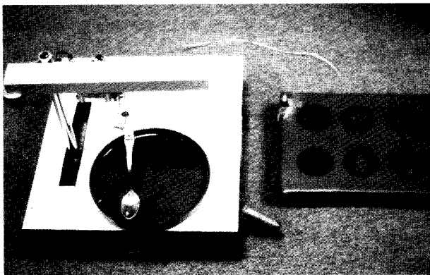
Figure 12.9. View of the Adapted Feeder and Control Panel.
