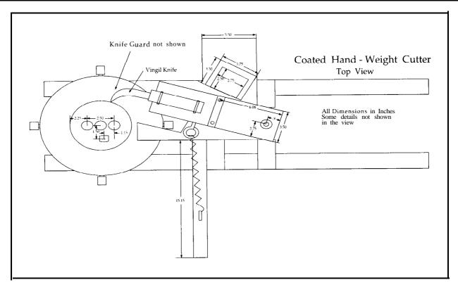
Figure 13.4. Coated Hand-Weight Cutter Top View.
