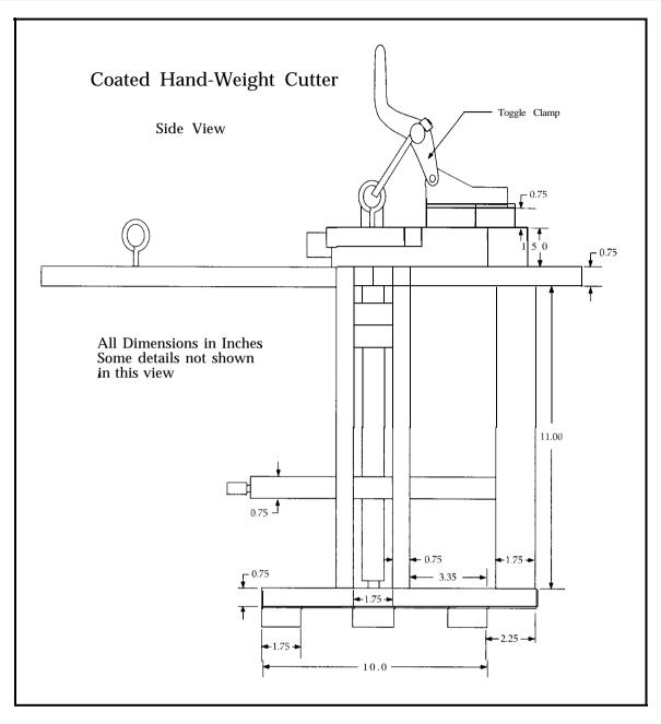
Figure 13.6. Coated hand-weight cutter side view
