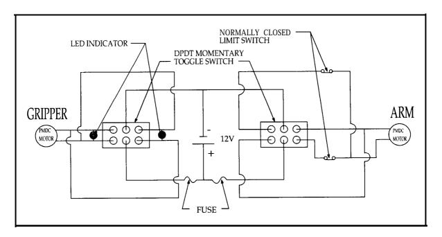
Figure 20.4. Wiring Schematic for Reacher/Gripper Device.
