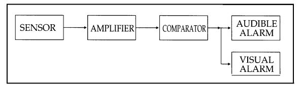
Figure 22.1. Block Diagram of Heat Sensor and Alarm.
