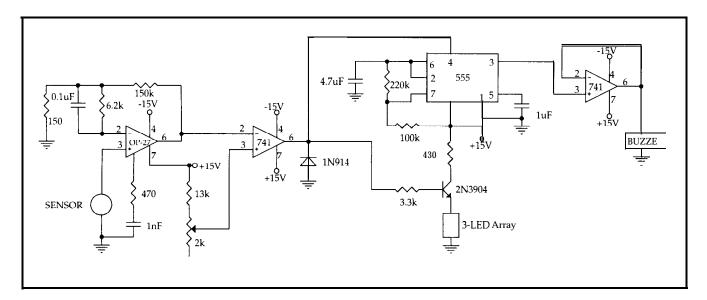
Figure 22.2. Circuit Diagram of Heat Sensor and Alarm.
