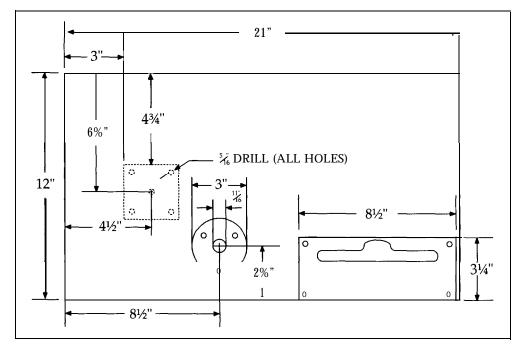
Figure 10.3. The Top View of the Flutophone Assembly Unit.
