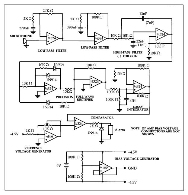
Figure 19.3. Schematic for the Speech Volume Training Tool.
