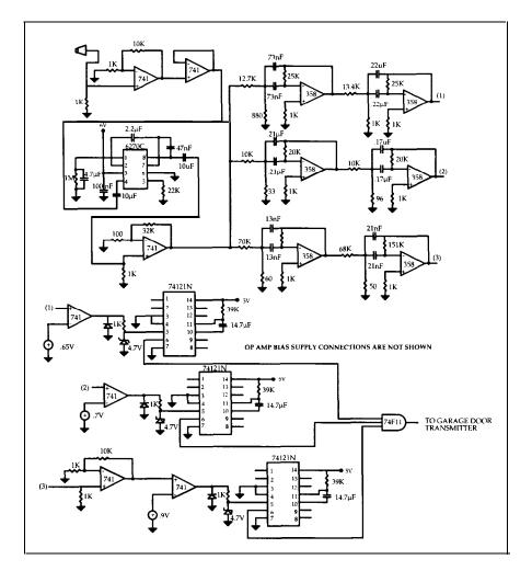
Figure 19.2. Schematic for the Voice Activated Door Opener.
