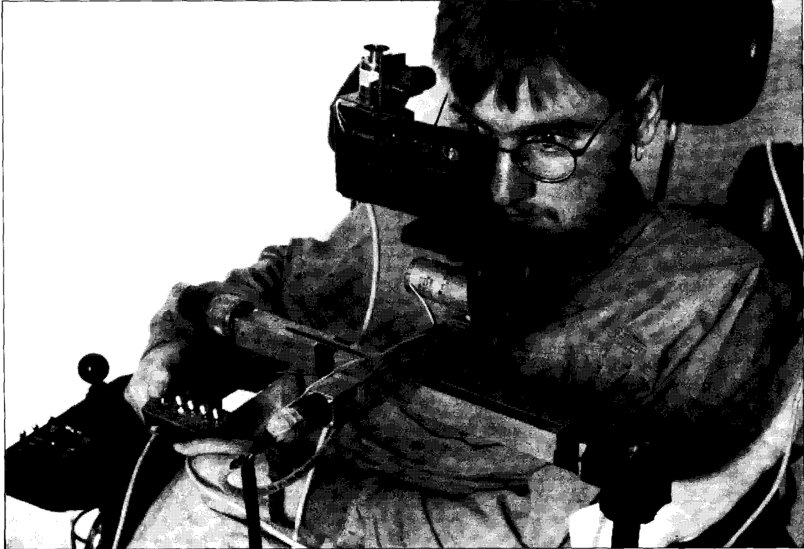
Figure 7.3. Wheelchair-Mounted Camera Control Mechanism.
