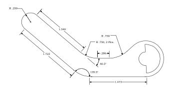
Figure 10.9. Geometrical Deta is Of Thum b.
