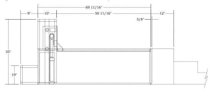
Figure 10.13. DesignConcept for the W heelcha in Lift.
