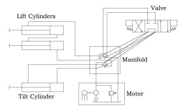
Figure 10.4. Flow Diagram Of The Hydraulic System.
