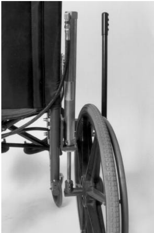
Figure 7.31. Close-Up Of Cylinder, Corrector, and Rear Wheel.
