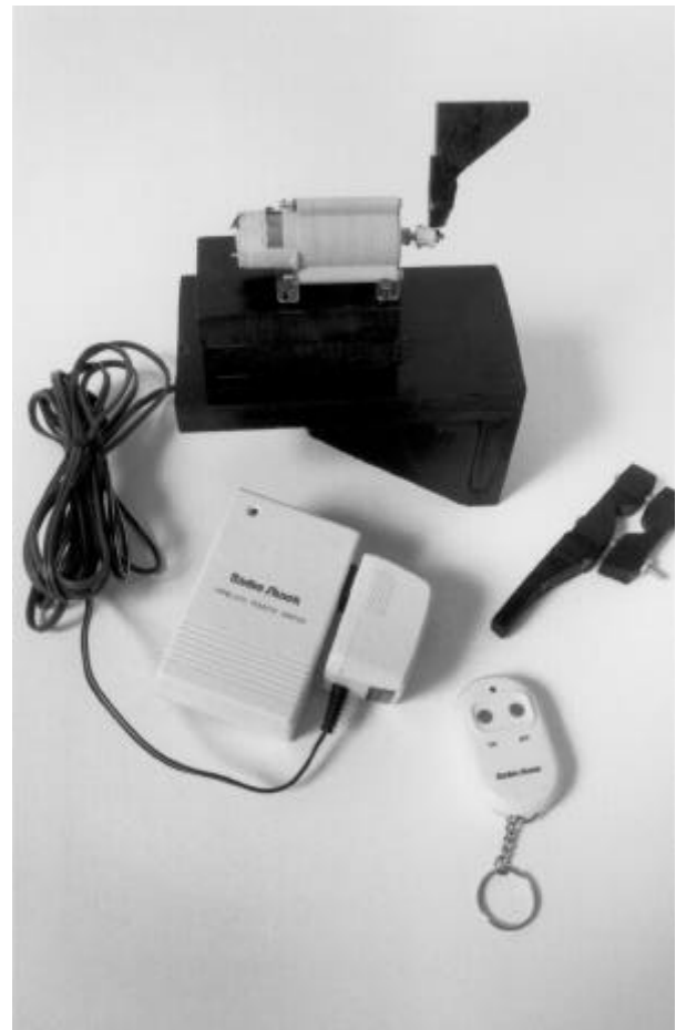
Figure 7.9. Door Opener Components.
