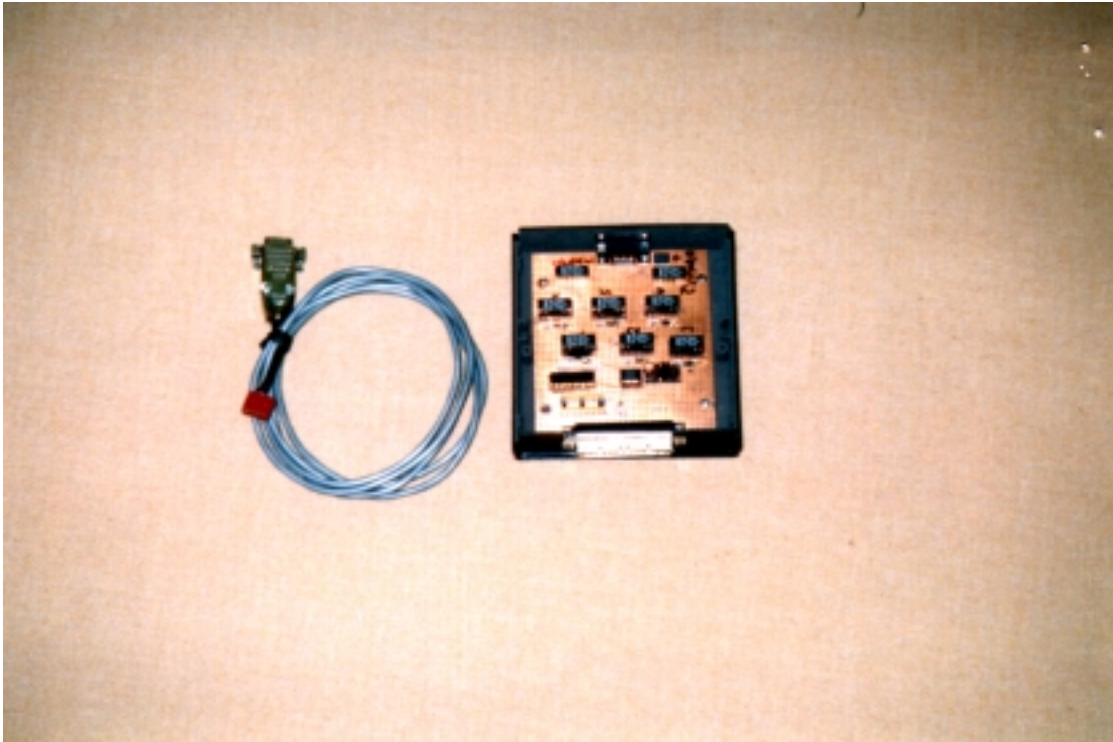
Figure 14.5. Computer Interface for Hospital Bed Control.
