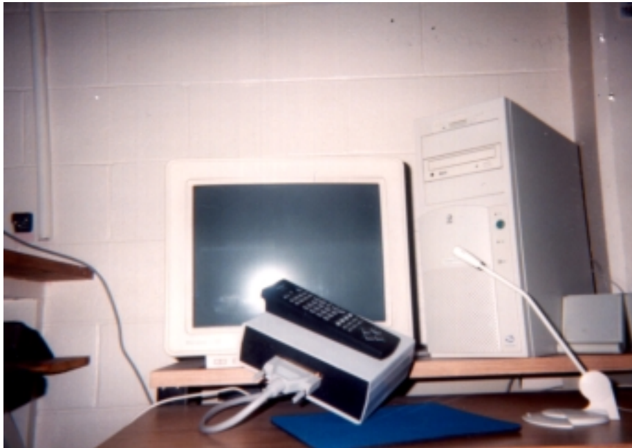
Figure 14.4. Voice Activated Environmental Control Unit.
