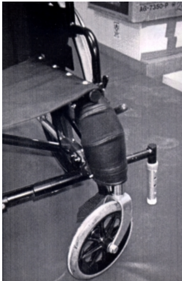
Figure 18.8. Adaptation to Eliminate Sharp Edges.
