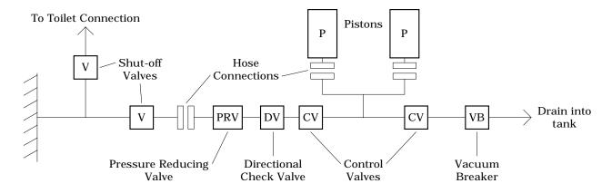
Figure 19.4. Plumbing Diagram.
