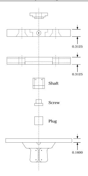
Figure 19.8. Assembly of Prosthetic Alignment Device.
