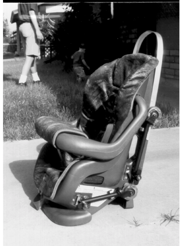
Figure 3.4. Side View of Stroller with Wheels in the Folded Position.
