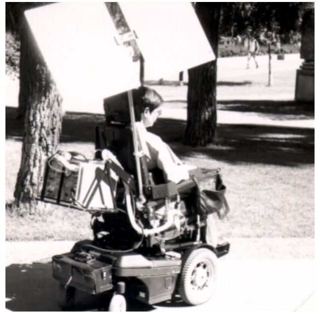
Figure 3.13. Rear View of Sunseeker, Showing Method of Attachment to Wheelchair.
