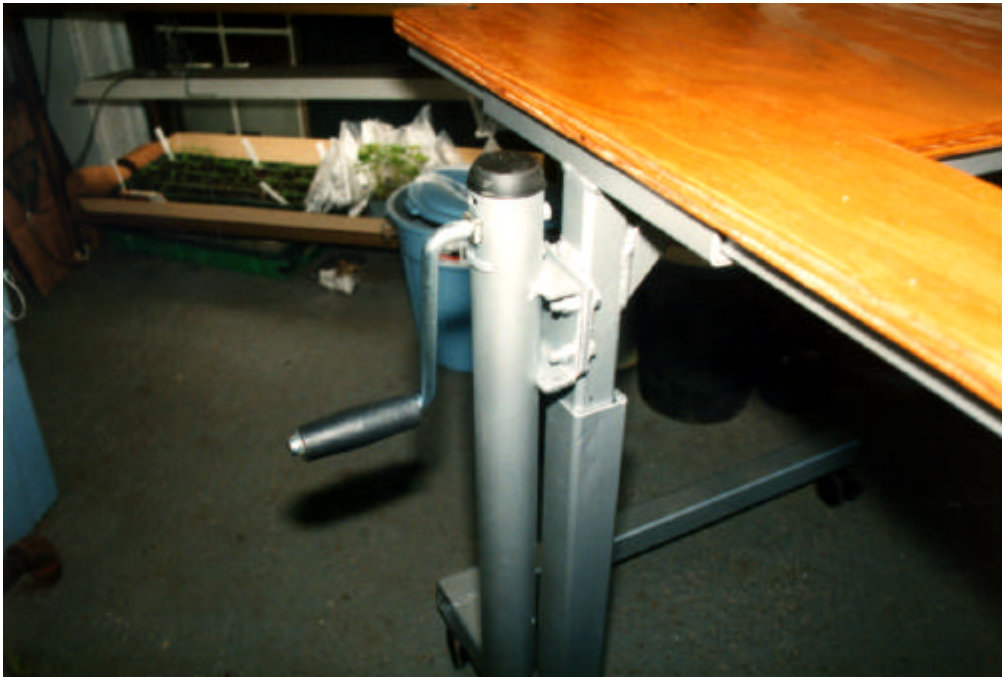
Figure 6.17. Close-up of the Crank and Jack Mechanism.
