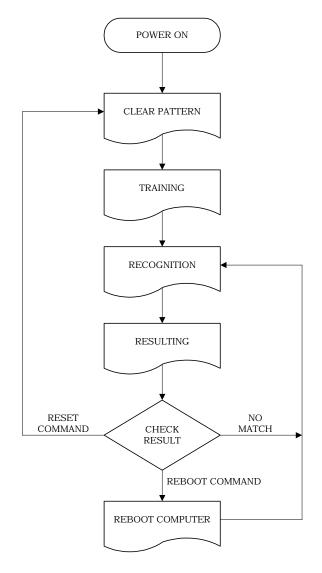
Figure 7.2. Block Diagram of the Operation of the System.
