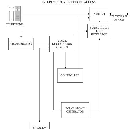
Figure 7.3. Block Diagram of the Interface for Telephone Voice Access.
