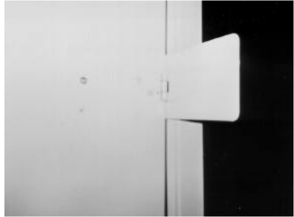
Figure 12.17. Installed Refrigerator Door Adaptation.
