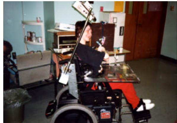
Figure 19.9. A Switch Driven Motor Controlled Arm for Positioning a Communication Device on a Wheelchair.
