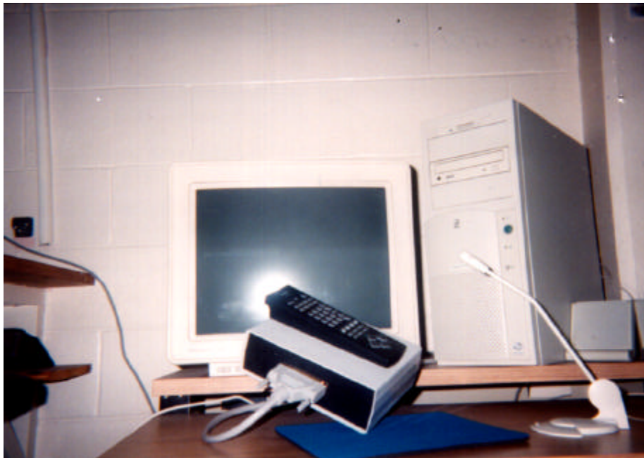
Figure 14.4. Voice Activated Environmental Control Unit.
