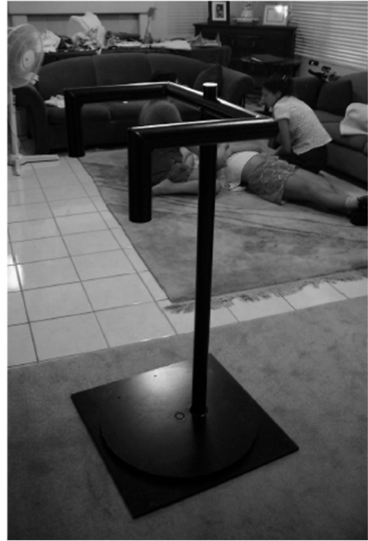
Figure 4.8. Transfer Device Including Turntable and Sturdy Frame.
