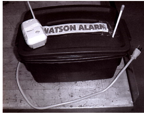
Figure 5.3. Base Unit and Handheld Receiver.
