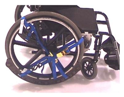
Figure 7.6. Wheelchair Ice Skates Attached to Standard Wheelchair.
