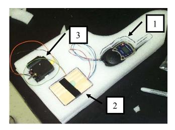
Figure 7.4. Inside of Life Vest: (1) Walkie-Talkie, (2) Circuit Board, (3) Vibration Device.
