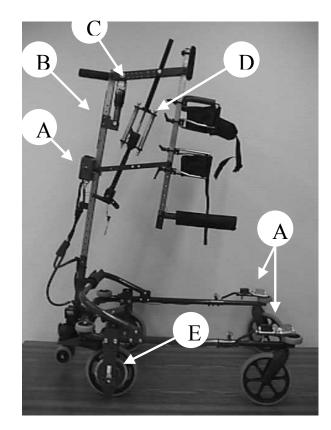
Figure 7.8. Walkabout 2A with modifications: A) Reward System, B) Digital Level (not shown), C) Damper, D) Spring Preload System, E) Braking System.
