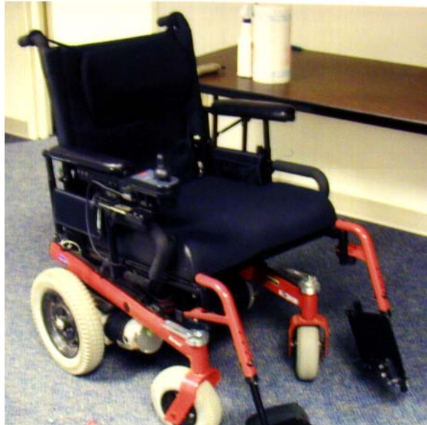
Figure 17.37. Front Wheel Controller Attached to the Wheelchair.
