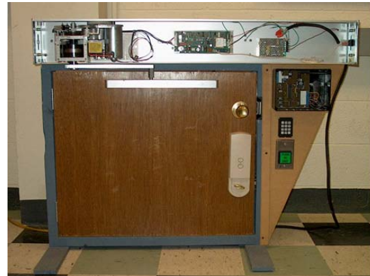
Figure 17.1. Automatic Door Opener.
