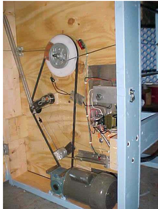
Figure 7.2. Inside of Rear of Chair, with Pulley (Upper Left) and Motor (Lower Right).
