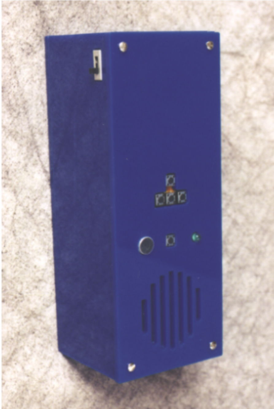
Figure 11.2. Digitally Secured RF Controlled Outlet.
