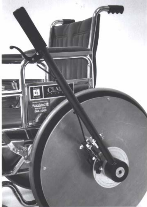
Figure 13.35. Close-Up of Handle Assembly.
