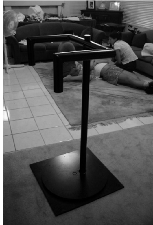
Figure 4.8. Transfer Device Including Turntable and Sturdy Frame.
