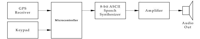
Figure 10.5. Block Diagram for the GPS Voice Output
