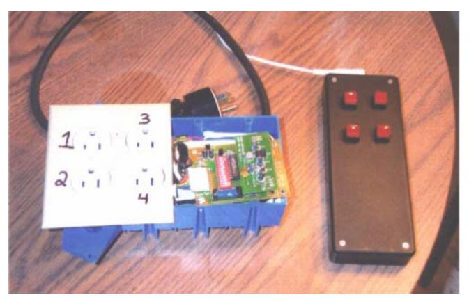
Figure 11.3. Digitally Secured RF Controlled Outlet.
