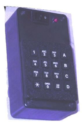
Figure 11.1. Switch Activated Voice Controller.
