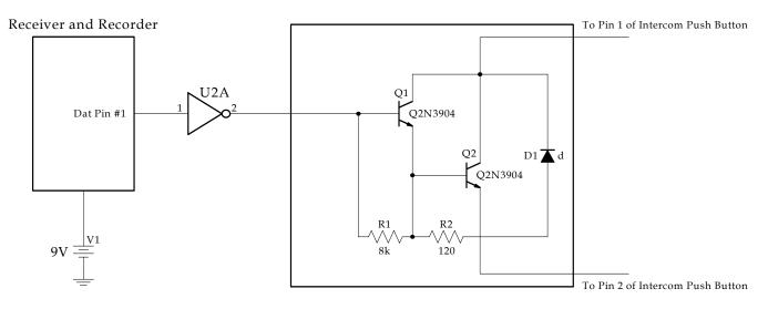
Figure 11.4. Schematic of Wireless Keyless Entry for Connection to an Intercom System.
