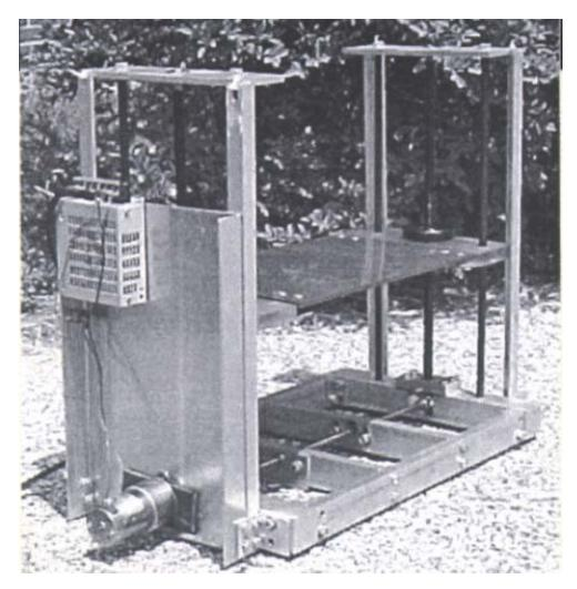
Figure 14.6. Portable Wheelchair Lifter.
