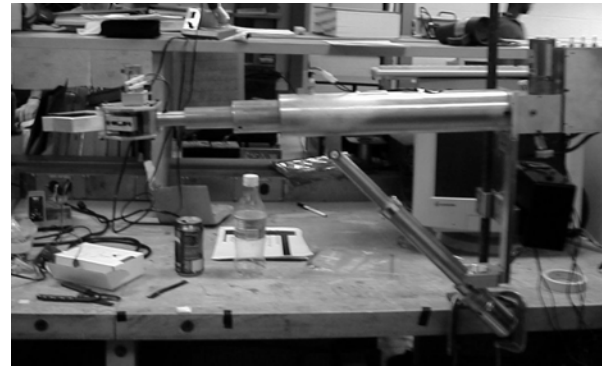
FIGURE 17.29. Object Retriever with Linear Actuator for Vertical Motion.
