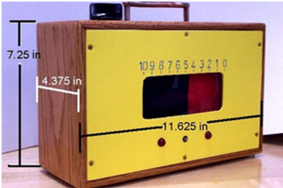
Figure 22.9. Dimensions of the Secondary Timer.
