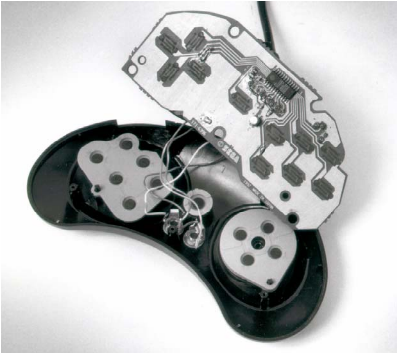
Figure 12.2. Circuit Connections Inside the Controller.
