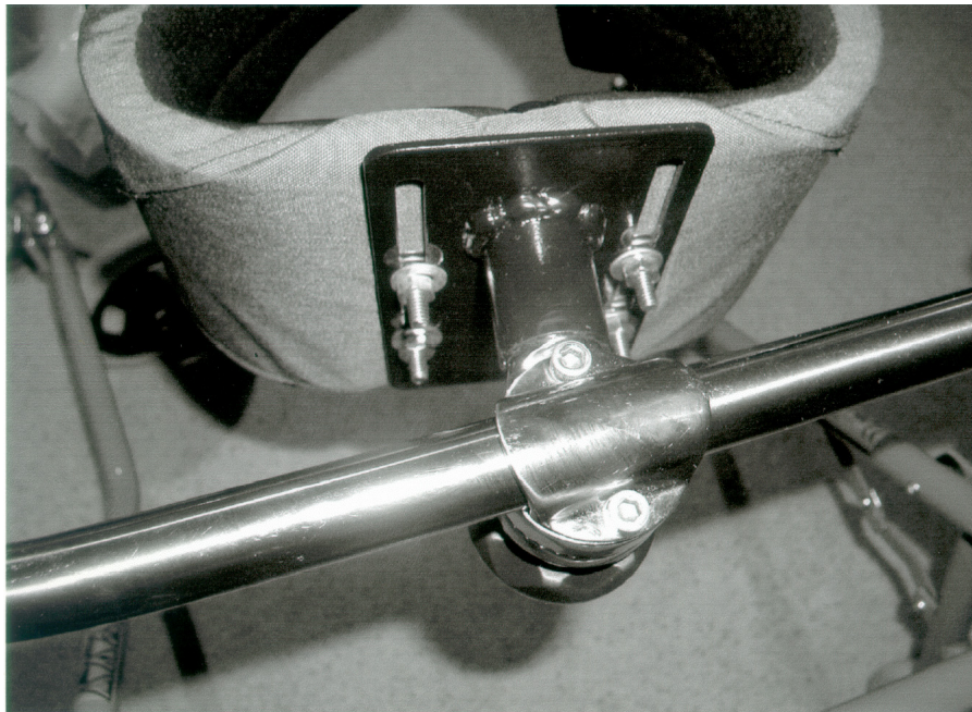
Figure 7.2. Slotted Back Plate and Rotational Hip Support.
