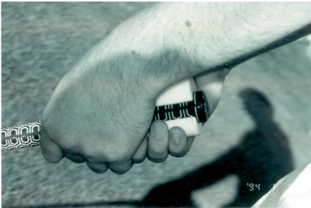
Figure 6.2. The Gripping System Attaches to a Standard Club while Maintaining a Typical Golf Grip.
