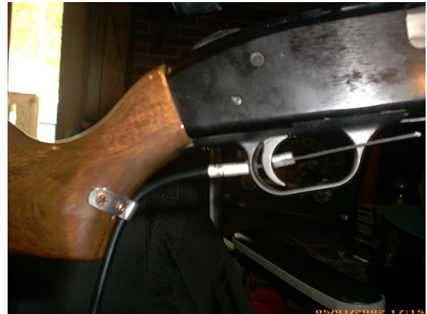
Figure 20.7. Cable Used to Pull Trigger.
