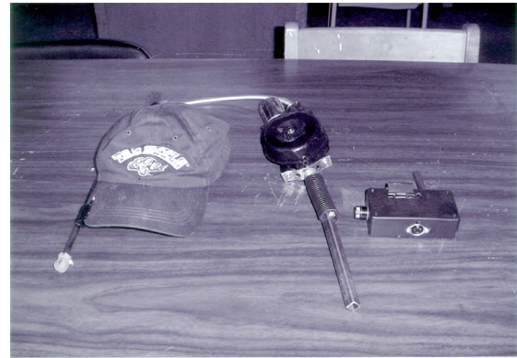
Figure 7.8. Retractable Head Pointer, Motor and Control Box with Switch.
