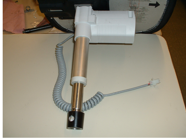
Figure 18.2: Low Noise DC Actuator and Coupling to AS.
