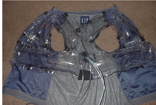
Figure 16.73. Air Containment Tubes on Deep Pressure Vest.
