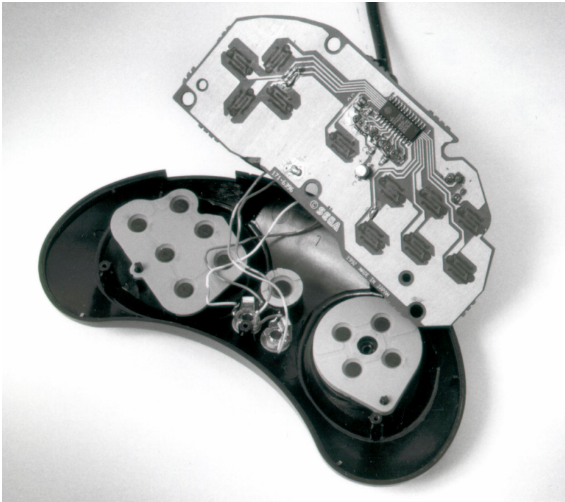
Figure 12.2. Circuit Connections Inside the Controller.
