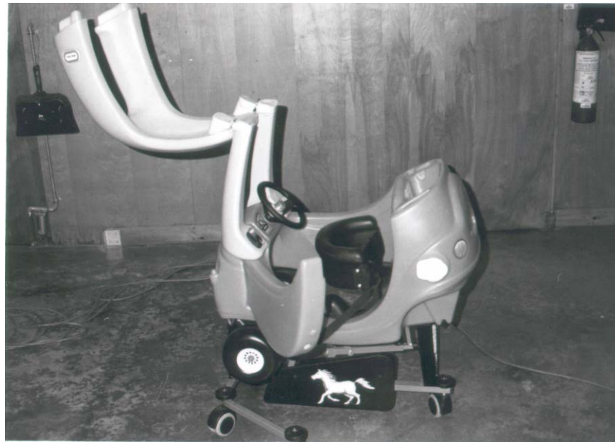
Figure 9.7. Retractable Roof on the Super Duper Cozy Coupe.
