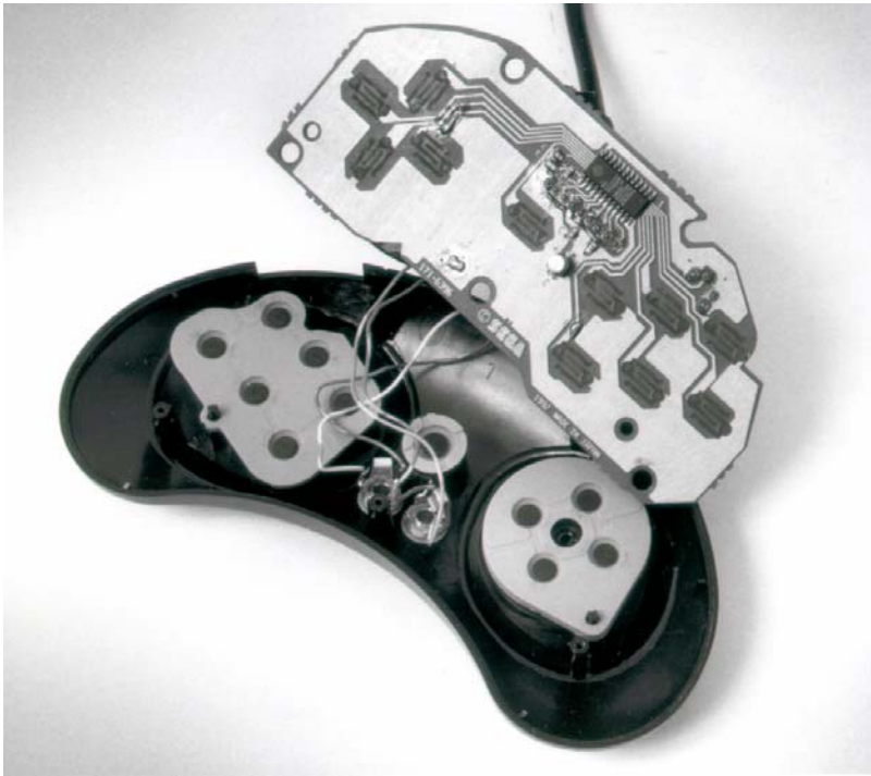
Figure 12.2. Circuit Connections Inside the Controller.
