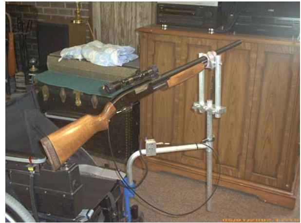
Figure 20.8. Turret Mounted on Wheelchair.
