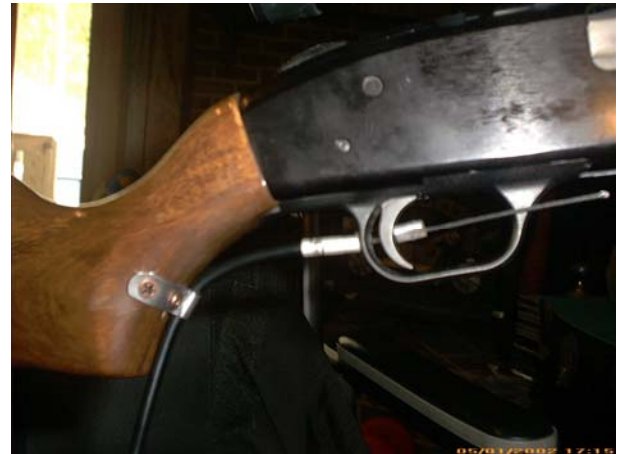
Figure 20.7. Cable Used to Pull Trigger.
