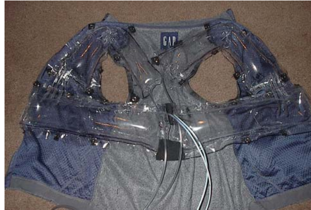
Figure 16.73. Air Containment Tubes on Deep Pressure Vest.
