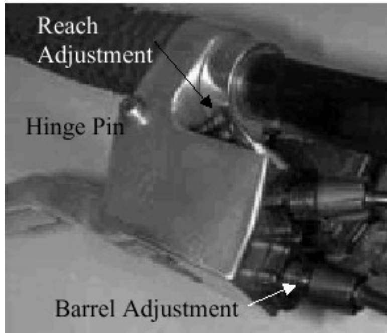
Figure 16.6. Barrel and Reach Adjustments.
