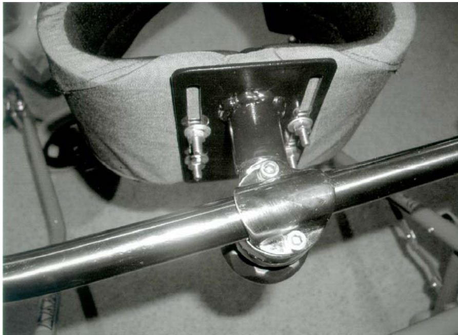
Figure 7.2. Slotted Back Plate and Rotational Hip Support.
