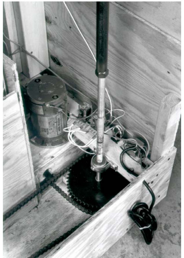
Figure 12.28. Motor-Chain Drive System.
