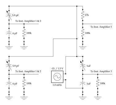
Figure 21.12. Circuit Design Implemented in Testing with the Capacitor Sensor.
