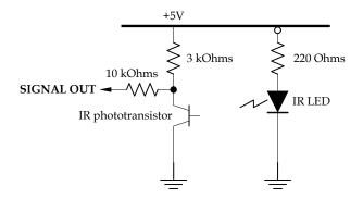
Figure 21.7. Circuit Diagram of Infrared LED and Phototransistor.
