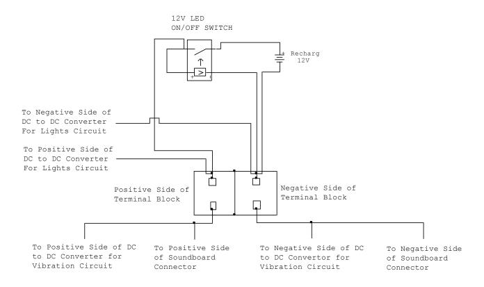
Fig. 20.11. Circuit Diagram of On/Off Switch and Terminal Board
