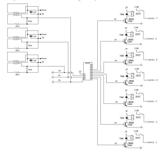
Fig. 20.6. Project Circuit Diagram.
