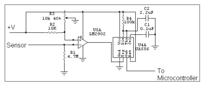
Fig. 20.3. Impact Detection Circuit.
