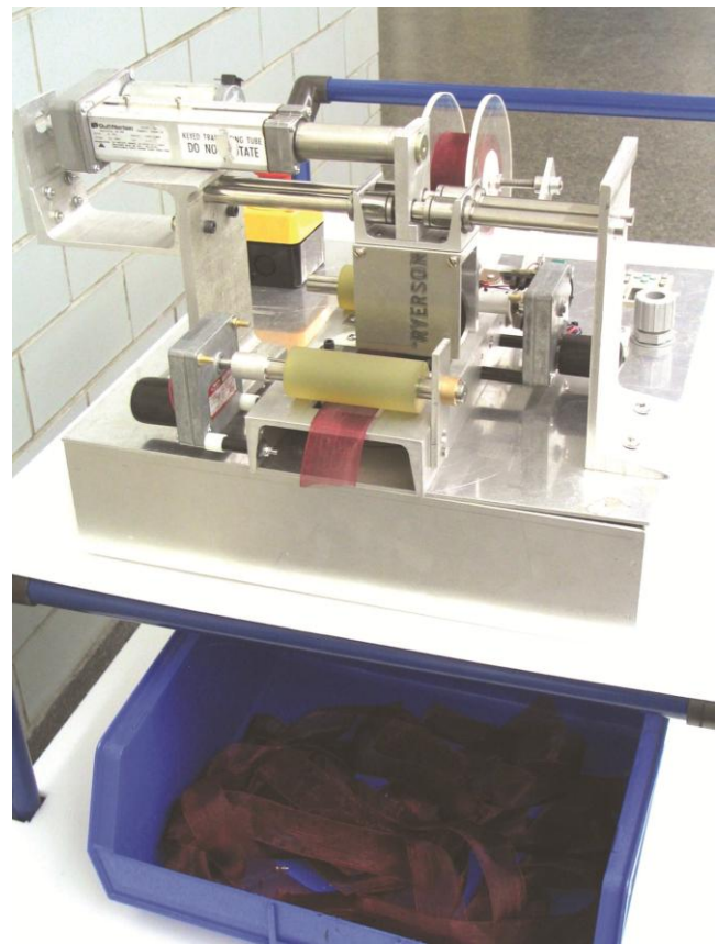
Fig. 20.3. A Close-Up View of the Ribbon Cutter mechanism. Cut Ribbon Falls into the Tray on the Middle Shelf.
