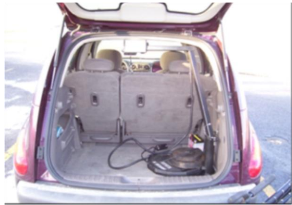
Fig. 18.5. Lift System in Closed Position.
