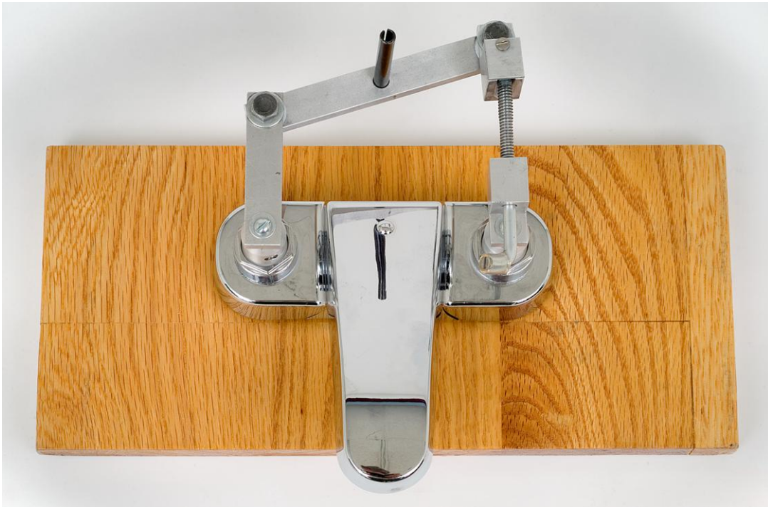
Fig. 11.86. Device with Adjusted Cold Water Tap.
