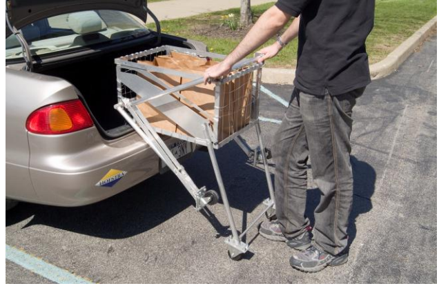
Fig. 11.102. Front Legs Collapse toward Rear as Cart is Pushed into Trunk
