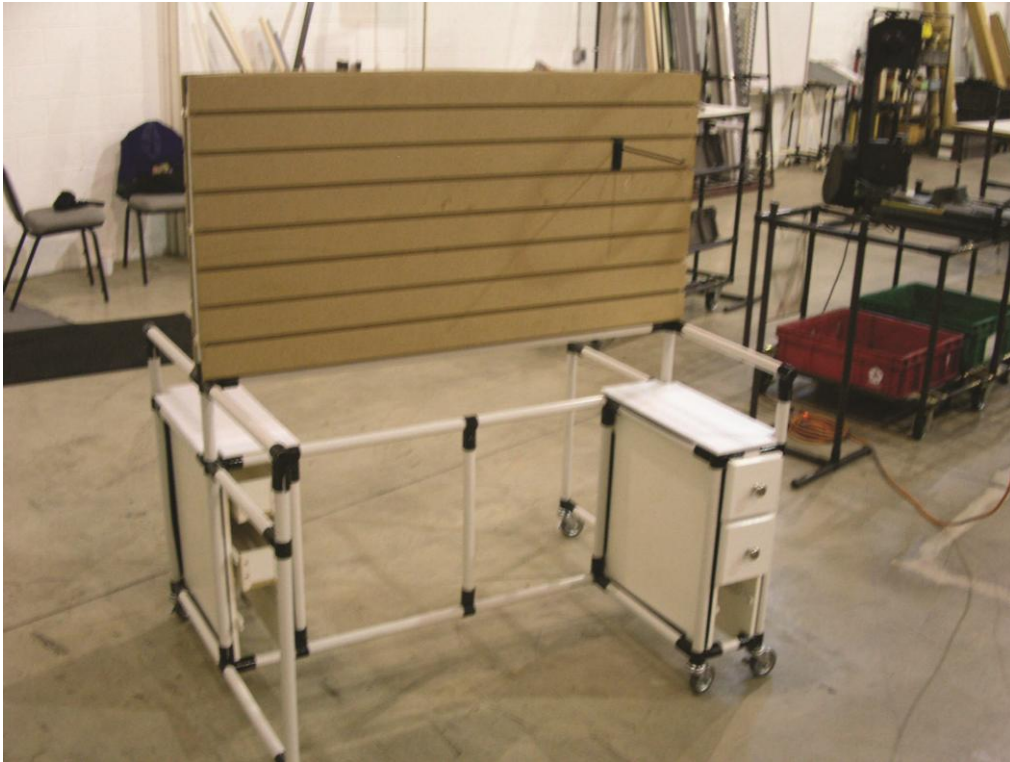
Fig. 20.4. New Creform Painting Workstation with Storage Drawers and Small Work Surface [Note Vertical Surface is Slatboard and Allows for a Variety of Tools to be Hung for Drying].
