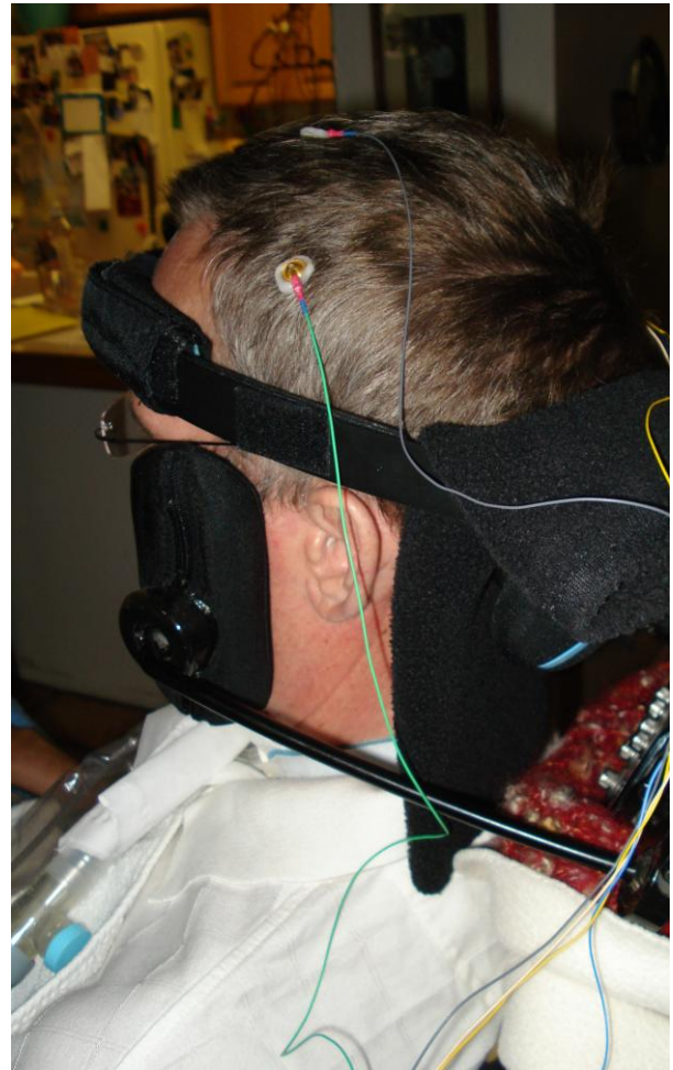
Fig. 6.4. Patient Wearing the EEG-Activated Alarm System.
