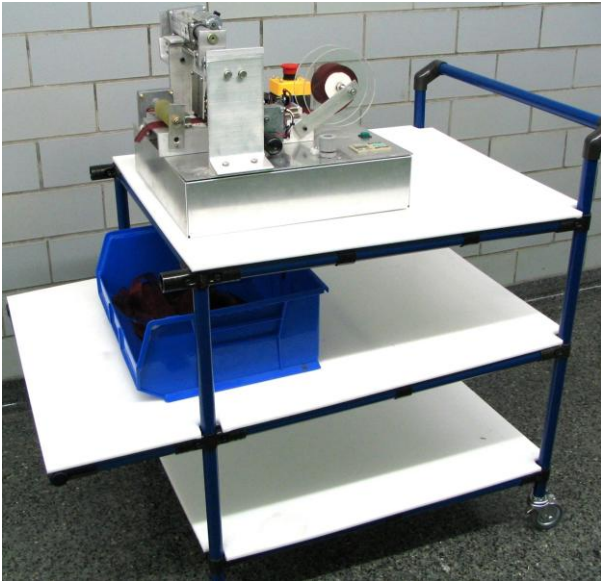
Fig. 20.2. Ribbon Cutter Mounted on Custom Mobile Cart (Note Yellow Emergency Stop Button (Red Cap) Behind Ribbon Cutter).
