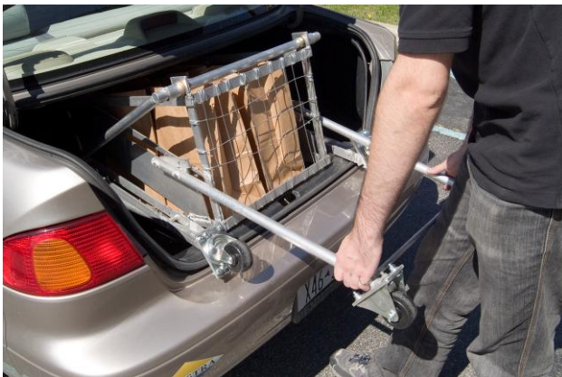
Fig. 11.103. Operator Slides Shopping Cart Rear Legs Forward.
