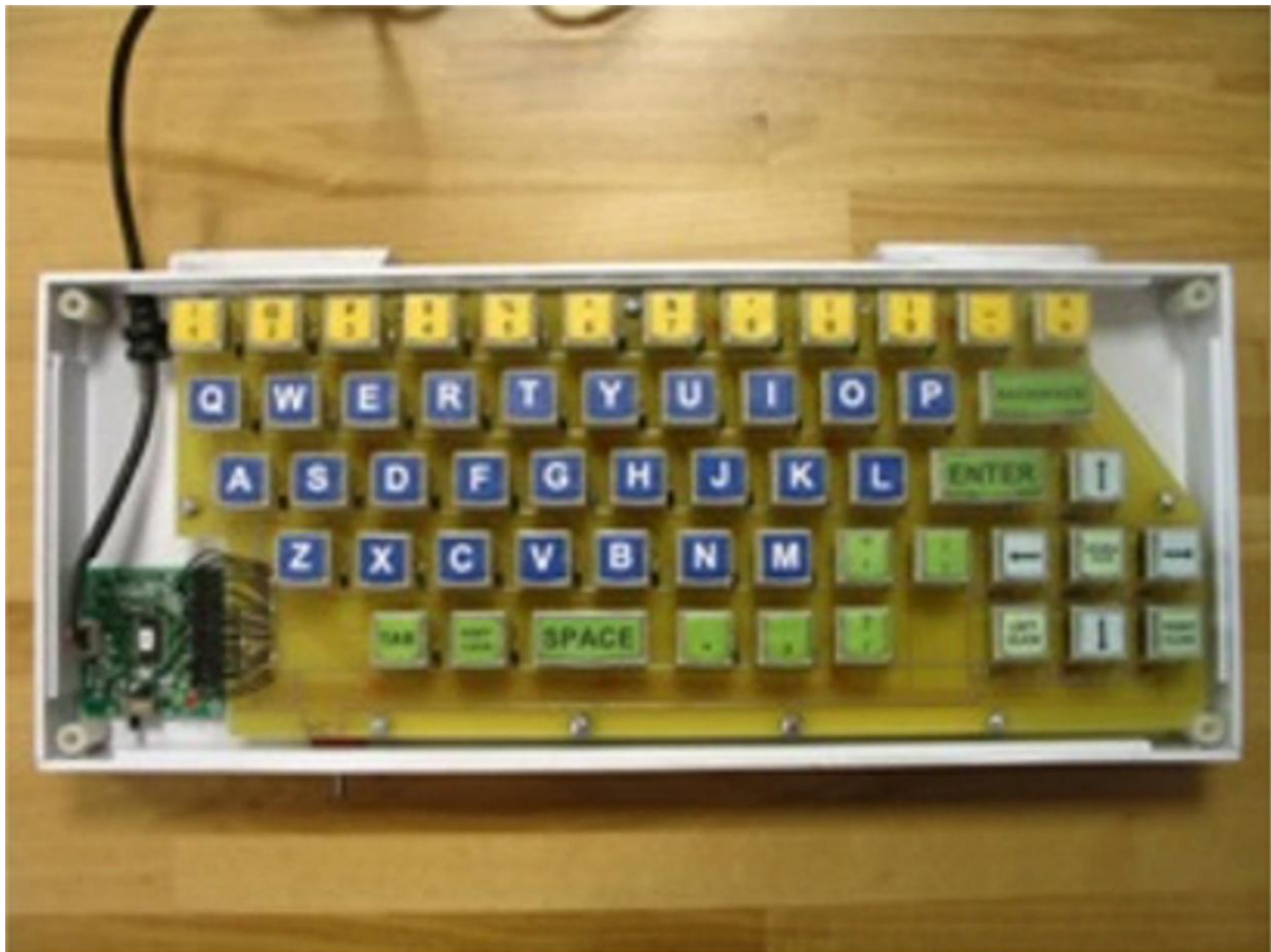
Fig. 14.3. Internal View of Keyboard.
