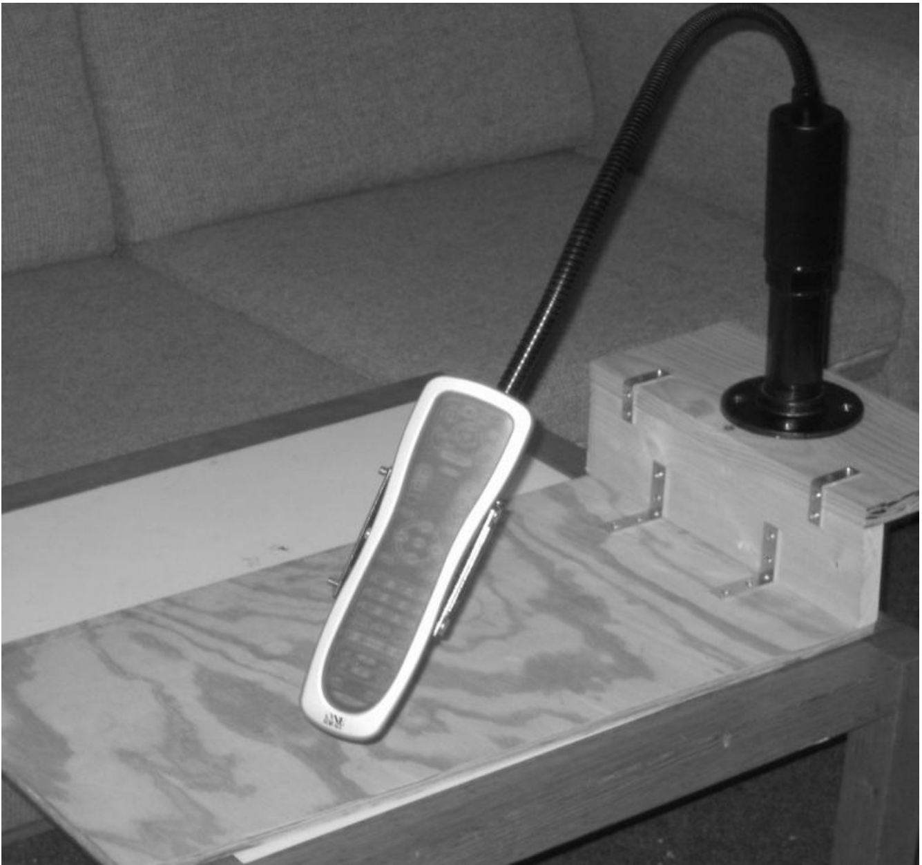
Fig. 9.5. The Remote Snake showing the basic configuration of remote, flexible extension, mounting, and base.
