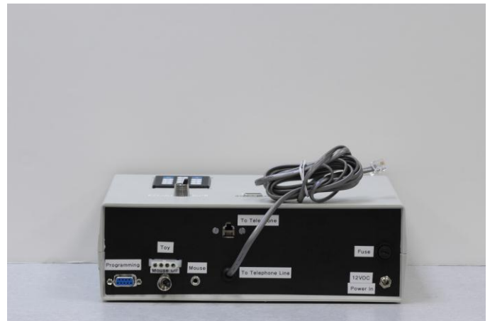
Fig. 12.20. Voice control system - rear view.
