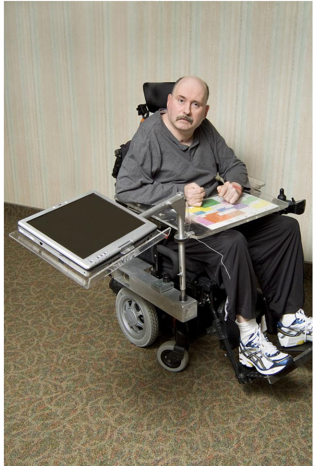
Fig. 8.46. Tablet mount swiveled out of the way of the user.
