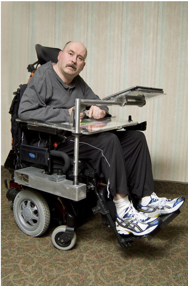
Fig. 8.45. Mount attached to wheelchair.
