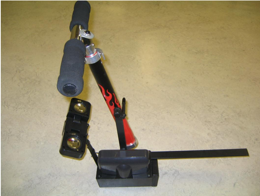
Fig. 13.9. Photo of the device. It mounts to the client's wheelchair by slipping the horizontal bar on the right side of the photo under the seat cushion. The client grabs the handles with both hands and pulls and releases the handlebar to count. The battery-powered circuitry is mounted in the black box at the bottom of the photo, and audio feedback is provided through the two speakers.
