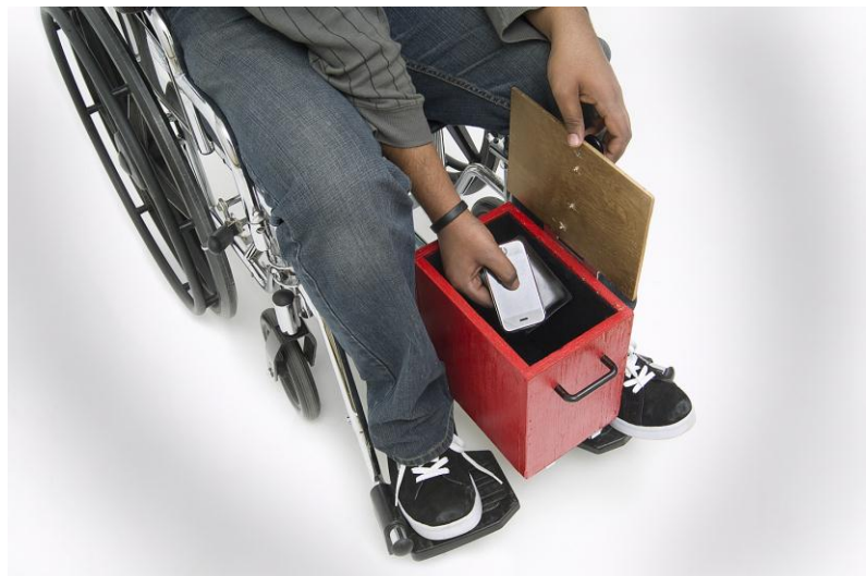
Fig. 8.91. Storage attachment opened and in use.
