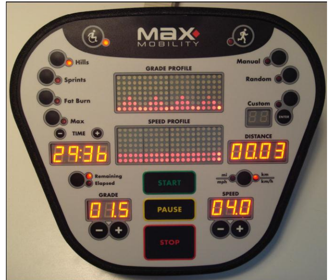
Fig. 15.2. The new treadmill control panel.
