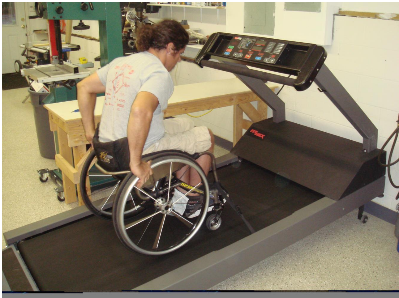
Fig. 15.1. The original wheelchair accessible treadmill prototype and control panel.
