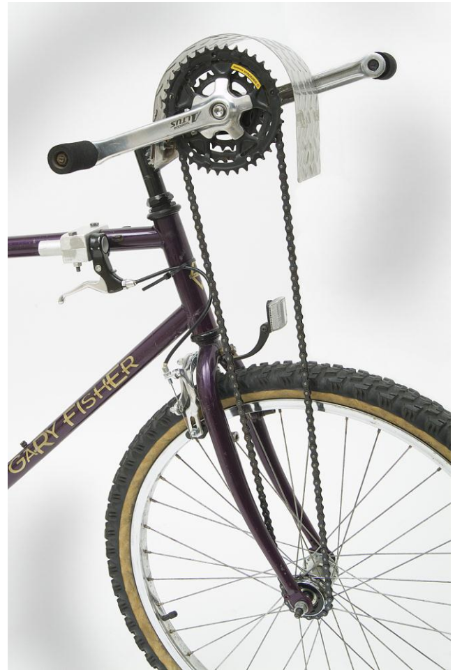
Fig. 8.93. Hand crank system with chain guard.
