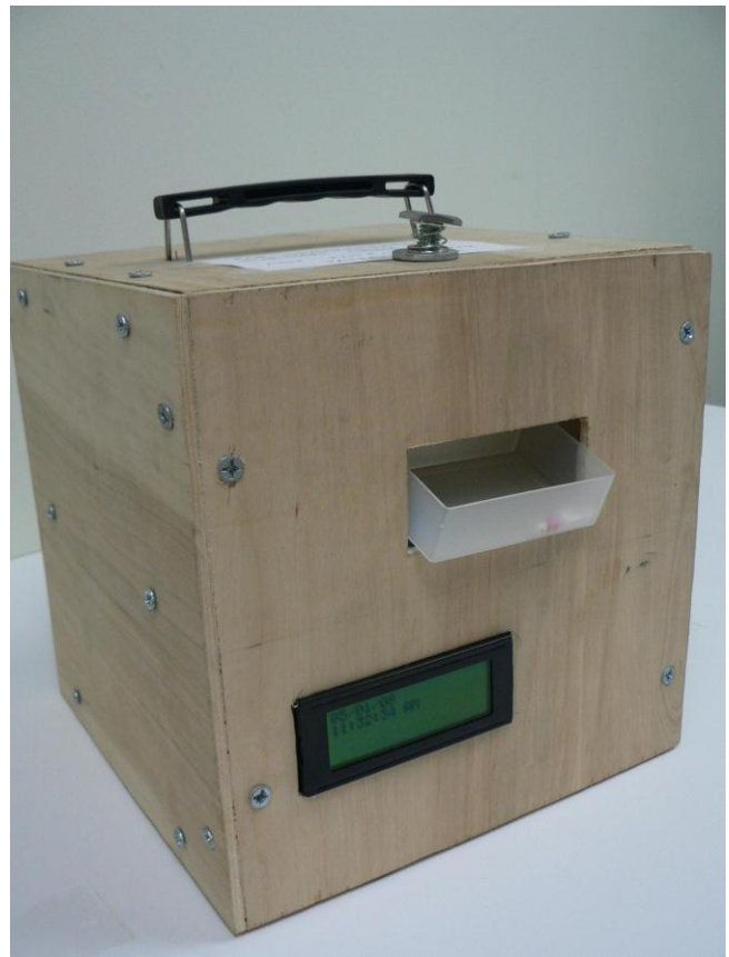
Fig. 9.8. Dispensing unit prototype showing carrying handle, pill punch control, output chute, and digital display.
