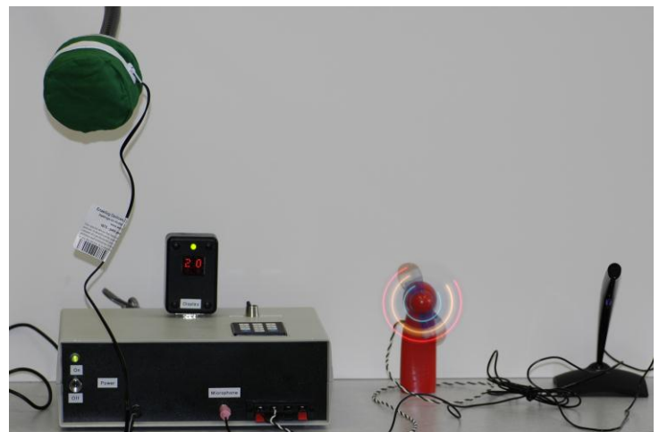
Fig. 12.21. Voice control system with pillow switch and fan.
