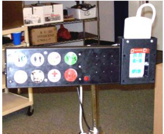
Fig. 9.1. The front view of the patient-nurse supplemental call system showing the large button display and hand-held call control caddy.
