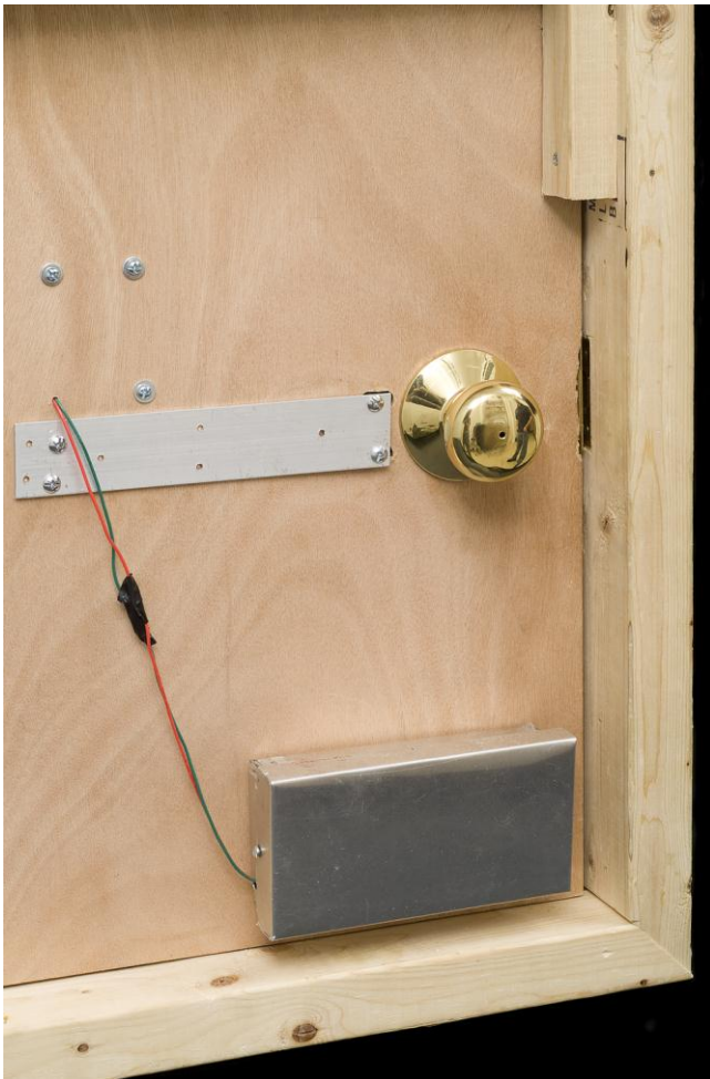
Fig. 8.34. Panel switch box.
