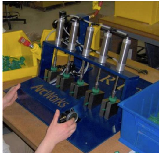
Fig. 7.23. Closure/straw adapter subassembly device in use.
