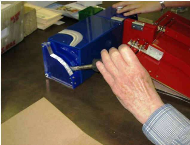
Fig. 13.4. The client is pulling the lever to dispense the next wafer seal, and then sticking the wafer seal onto the folded mailing.
