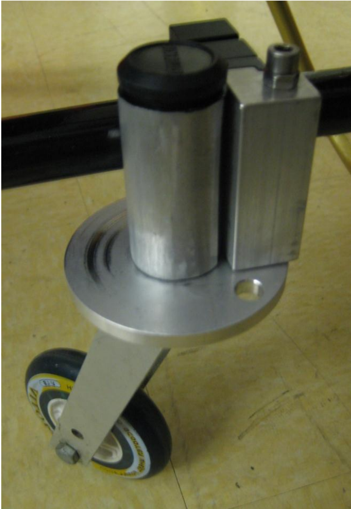
Fig. 15.8. Image of the cross-slope compensation mechanism.
