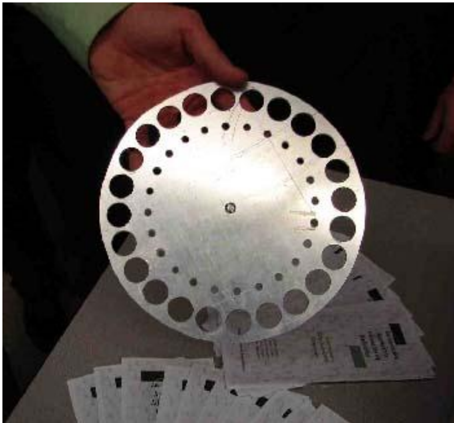
Fig. 9.9. Pill wheel showing 24 compartments and optical indexing holes.
