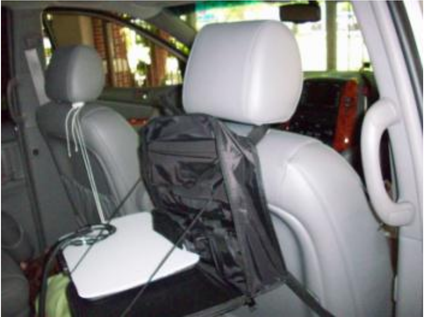
Fig. 9.11. The Video Window Viewer as installed in the client's family vehicle. The monitors are attached to the underside of the fold-down tray.
