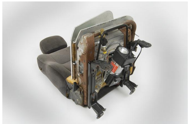
Fig. 8.77. Air compressor and hoses.
