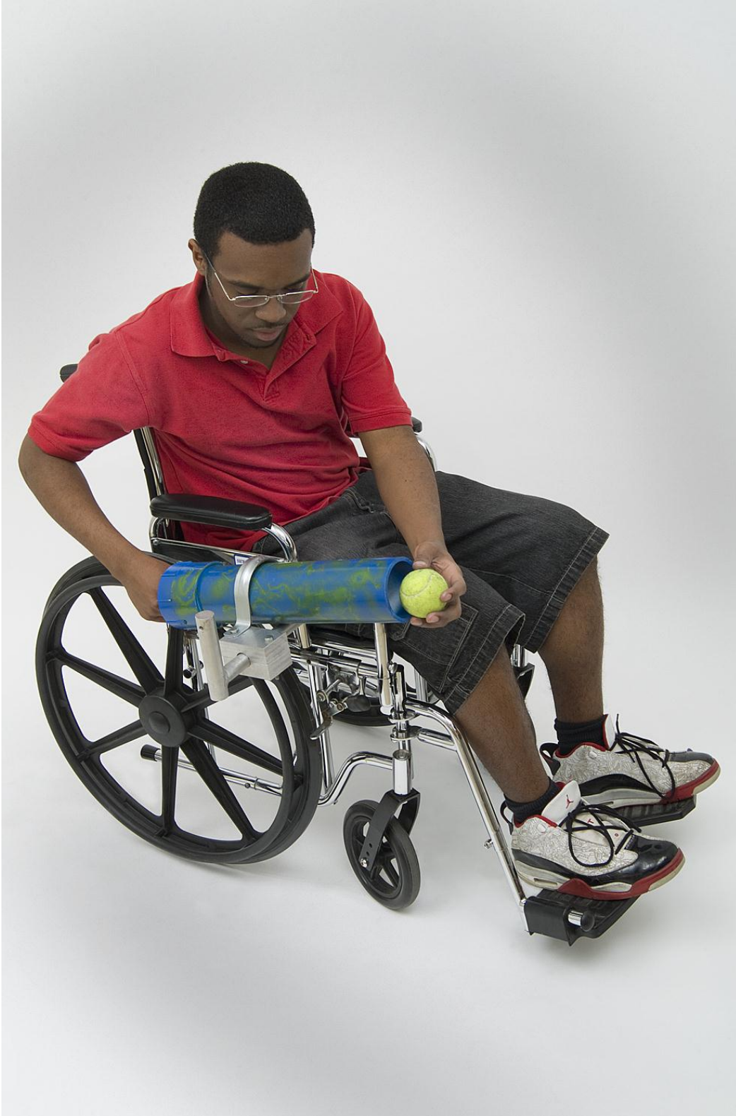
Fig. 8.48. Tennis ball launcher mounted to a wheelchair.
