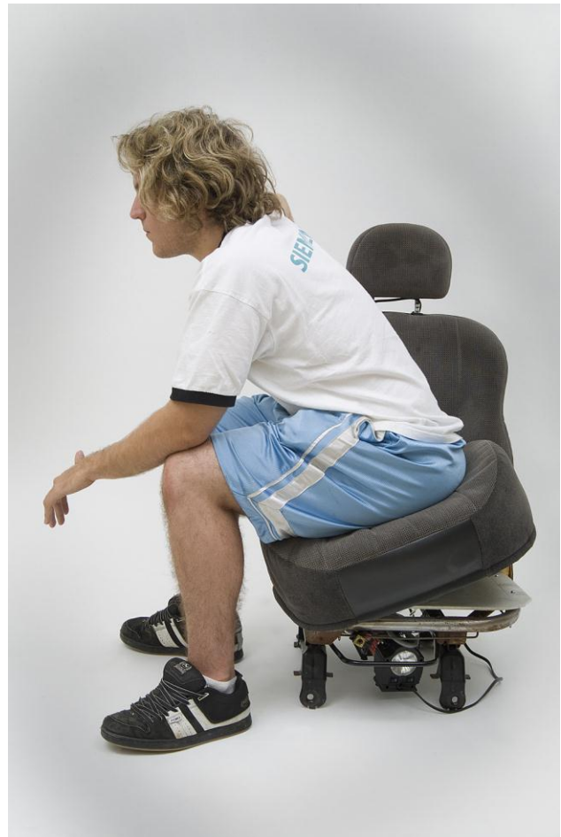
Fig. 8.76. Assist in standing car seat assisting the user.
