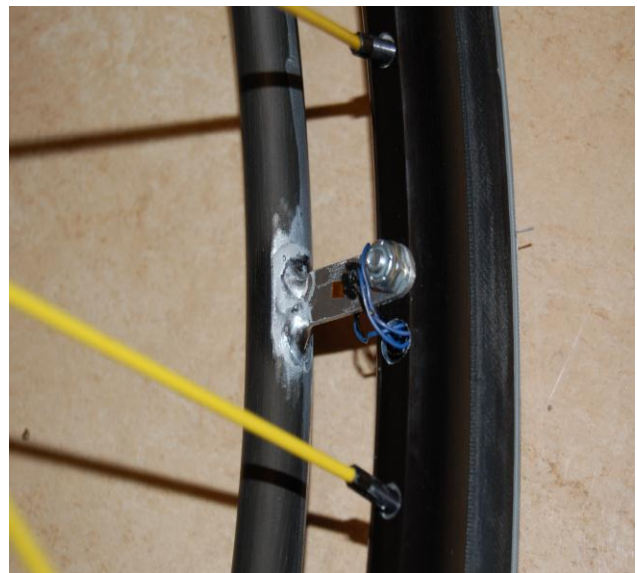
Fig. 15.5. Strain gauges attached to the push rim tabs.
