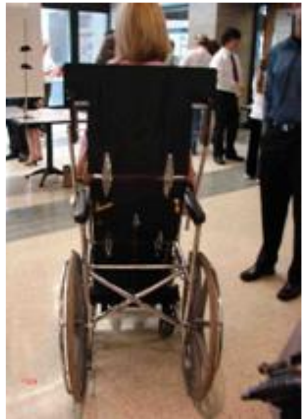
Fig. 9.12. The standing wheelchair. Top: wheelchair configuration. Bottom: standing configuration, rear view showing gas springs and 4-bar mechanism.
