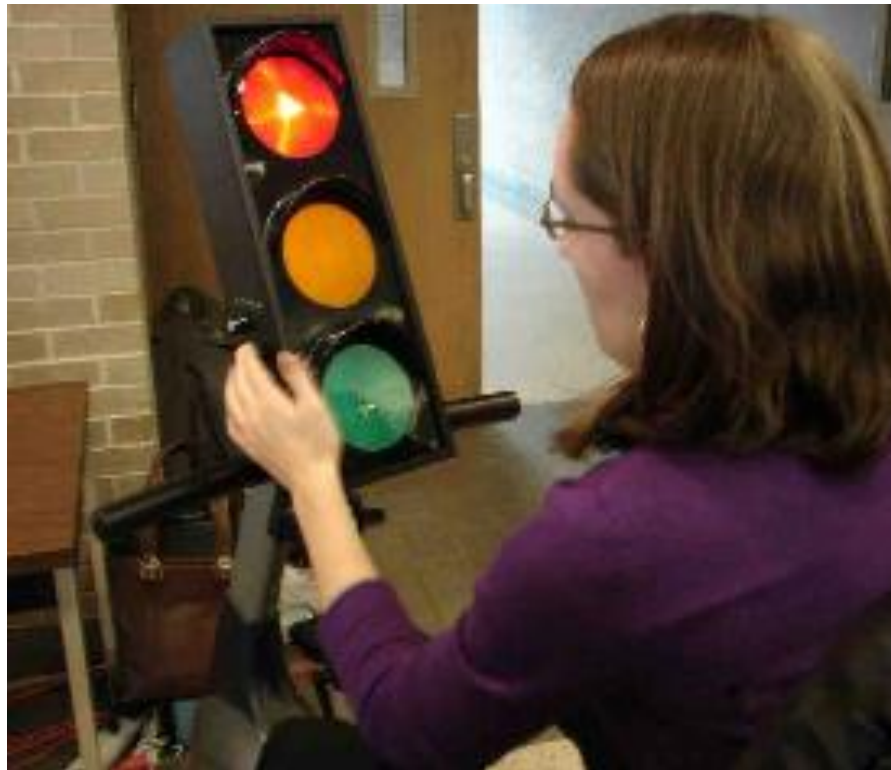
Fig. 9.7. The stoplight feedback unit. The five LEDs and the timer controller for the teacher is located above the left hand.
