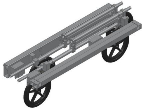
Fig. 6.8. Solid CAD model of collapsed UPF VI.
