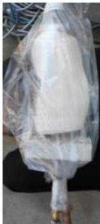
Fig. 6.27. Bag tightened around vacuum hose.
