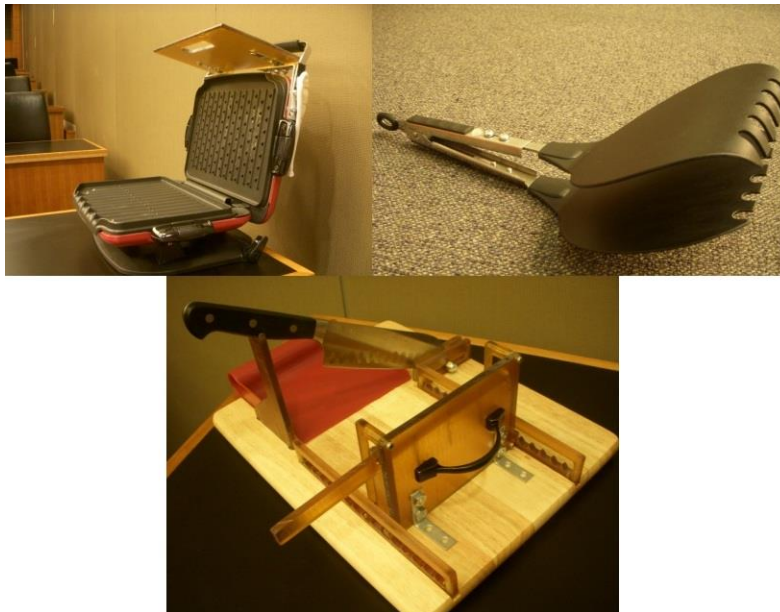
Fig. 7.16. Iron Chef Devices [clockwise from top left]: Modified Grill, Spatula/Tongs, and Cutting Device
