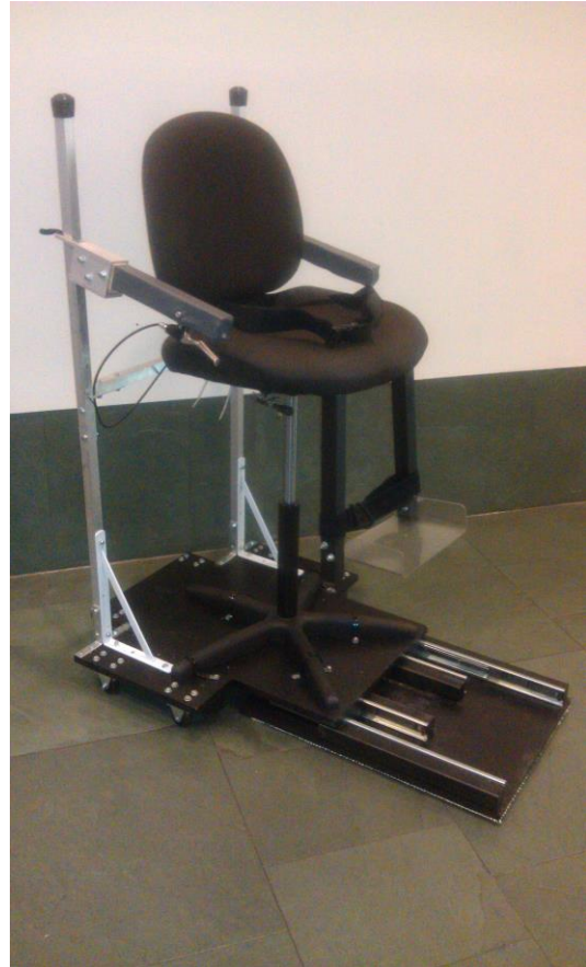
Fig. 7.21. Movin On Up Chair, raised position with base in open position.
