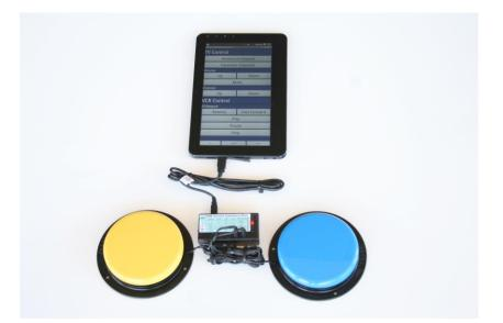
Fig. 9.7. Android Device with two button inputs.
