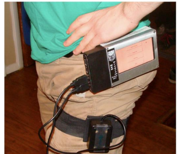
Fig. 12.26. Wearable, programmable base unit. Shown being used to capture knee flexion angles.
