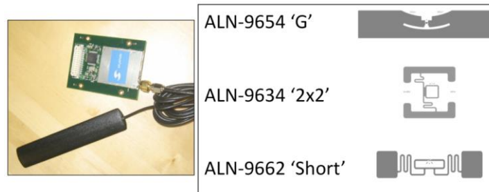
Fig. 12.9. Reader, antenna, and tags selected based on testing.
