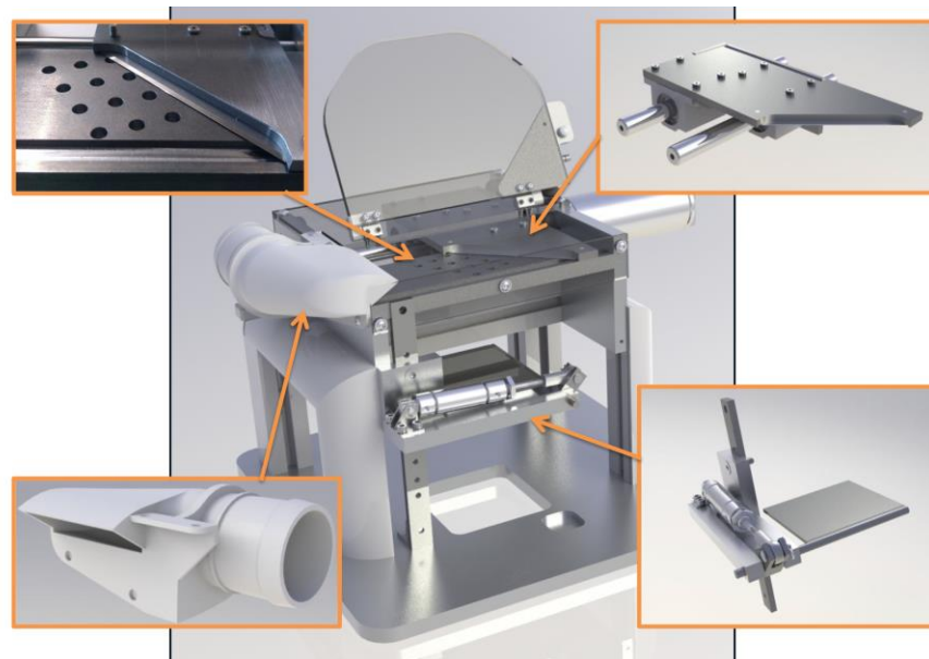
Fig. 12.21. Straw cutter design. Clockwise from top right: blade carriage, trap door/height adjustment, vacuum attachment, and cutting plate.
