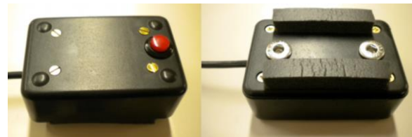
Fig. 12.29. Front and back of sensor unit with reset button, showing snaps to attach to knee or head straps.
