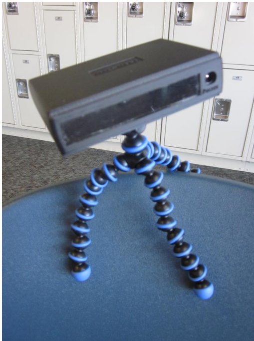
Fig. 12.17. Alert notification device, mounted on tripod without power cord and bed shaker.
