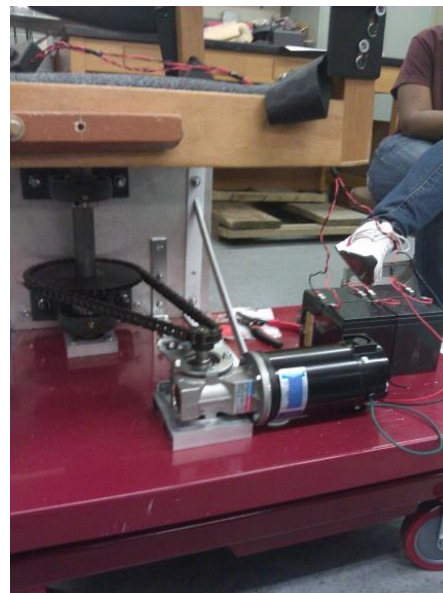
Fig.14. 8. Rotating Mechanism of Elevating Wheelchair Relocator.
