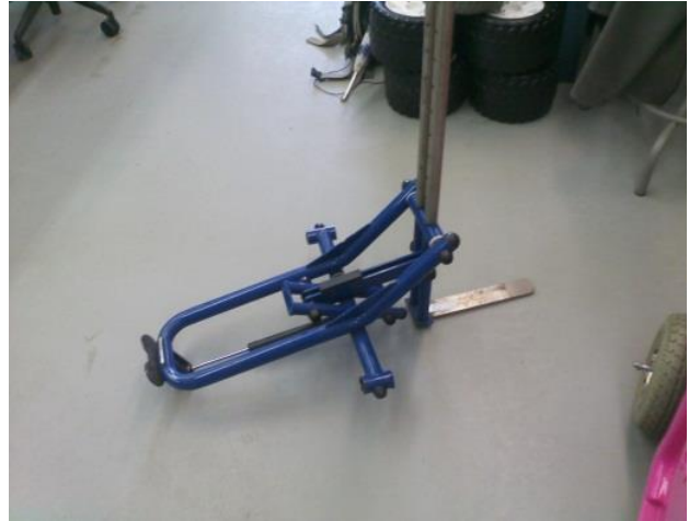
Fig. 17.19. TumbleForms TriStander after having the piston assembly isolated out.
