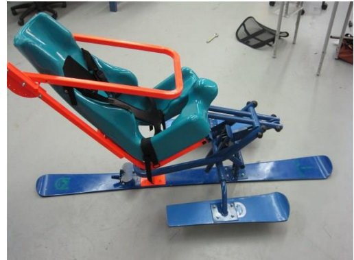
Fig. 17.17. The Assisted Skiing Device.
