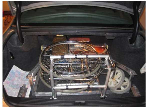
Fig. 20.21. Picture of the wheelchair on the unit inside the trunk of a car.
