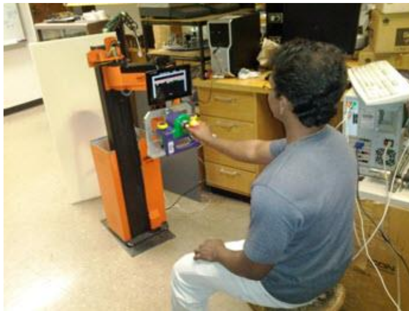
Fig. 23.1. (Top) CAD representation of MH5 and the generic end-effector holding the E-LINK. (Bottom) shows the completed generic bracket with display LCD and E-LINK mounted on an RT 100 robot. This robot is not suited for the clinical therapy sessions, but was used to verify the prototype generic fixture and E-LINK attachment.
