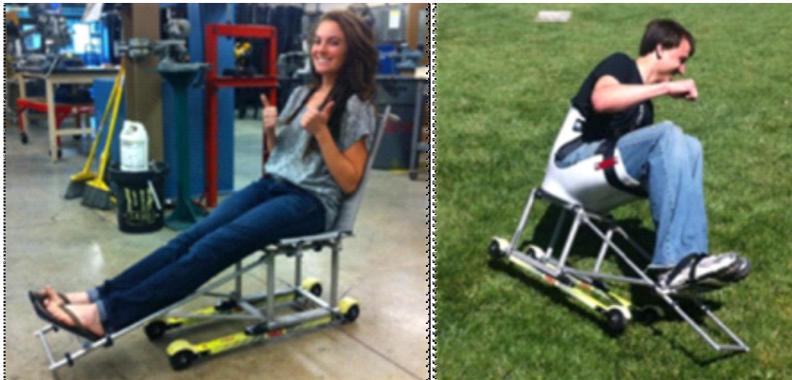
Fig. 6.14. Sit ski in two configurations – (a) bench seat and (b) bucket seat.
