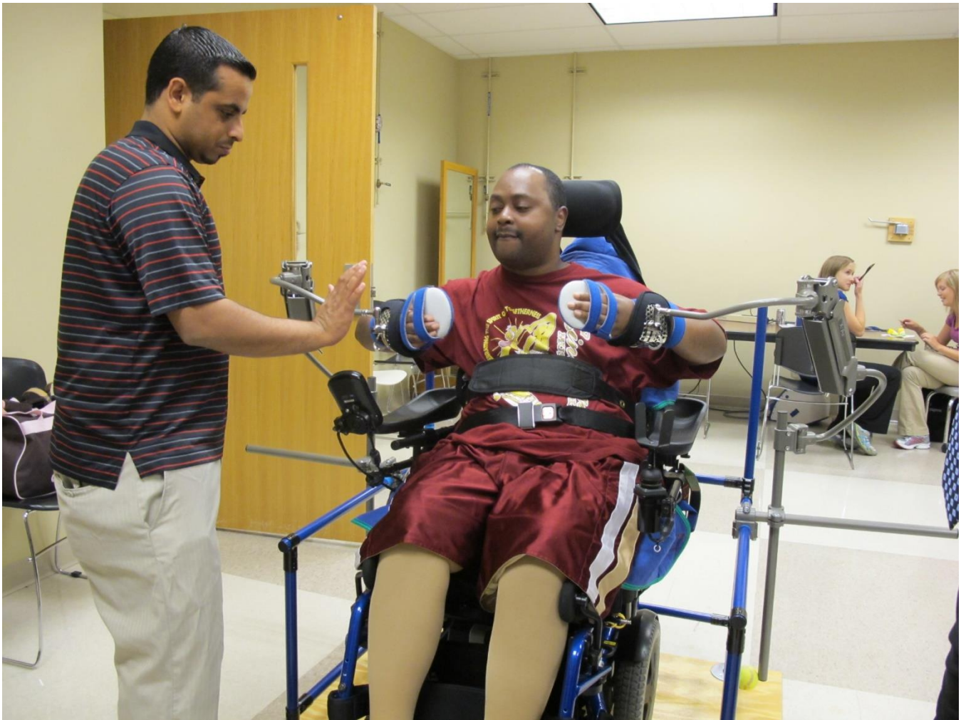
Fig. 23.8. A client using the xAr devices while sitting in his wheelchair in the Creform frame.
