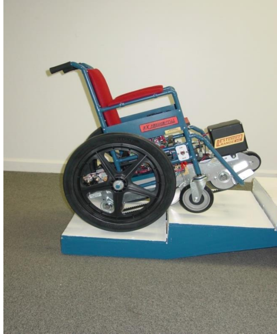
Fig. 8.13. The Proposed Wheelchair Allowing the Transport of a Person Up and Down Steps.
