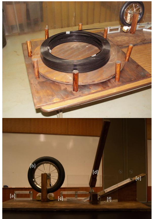
Fig. 7.21. The Cutting Edge Device: Above picture is the turntable and metal spool; Below picture is cutting device [a] First pipe guide [b] Rubber wheel flush on bed castor wheels [c] Second pipe guide [d] Extended lever arm [e] Sliding wooden ramp [f] Safety shield.
