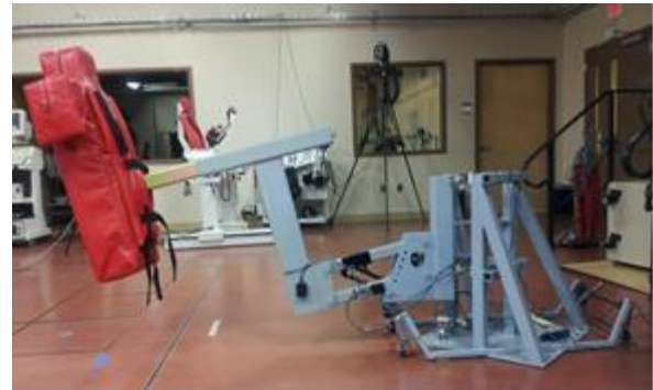
Fig. 15.16. Prototype of the Force Measurement System.
