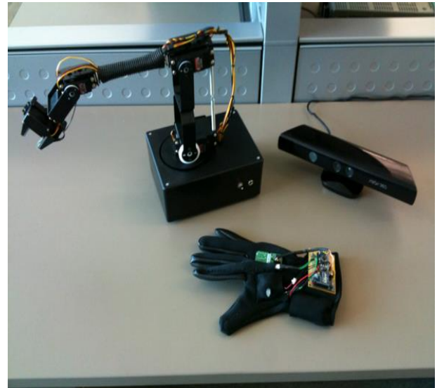
Fig. 8.14. Teleoperated Robotic Arm – System Components.
