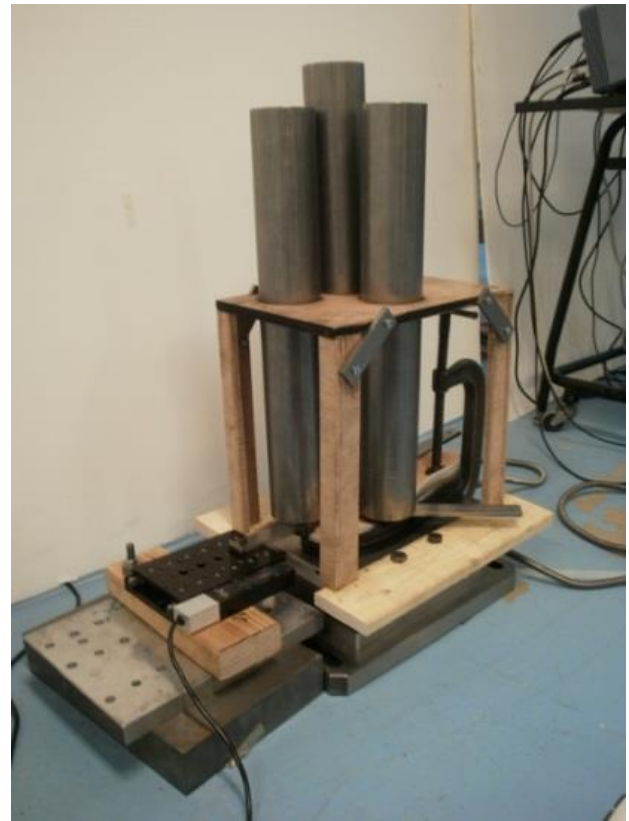
Fig. 18.9. Shear Test of Diabetic Insole Prototype.
