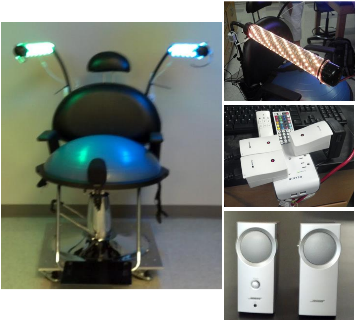
Fig. 16.3. The Balance Trainer (left) along with the LED lights and flexible gooseneck arms (top right), the wireless remote system (Middle Right), and the speakers (Bottom Right).
