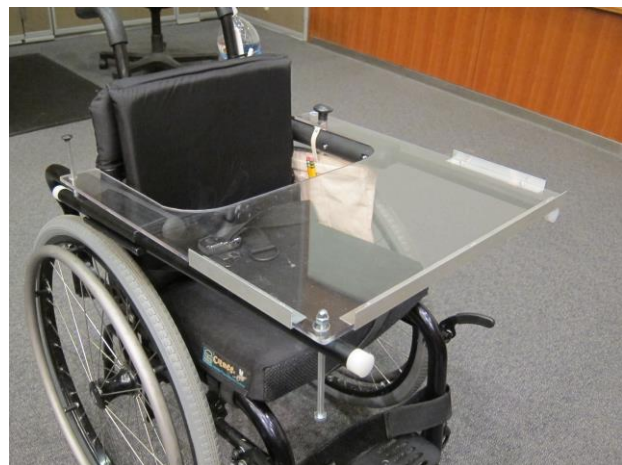
Fig. 7.17. (a) Shows the lap tray in the storage position on the right side of the wheelchair. This position still provides her access to the wheels so that she can propel her wheelchair. To use the lap tray, the client can slide the tray forward and swing it across the chair, putting it in the position shown in (b). The storage bag is located under the left armrest.
