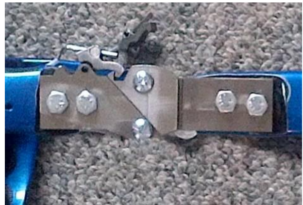
Fig. 12.14. A) The Final Brace Prototype. B) Close-up Image of the Replaced Knee Joint Mechanism.
