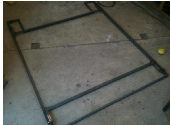
Fig. 9.13. Welded platform frame
