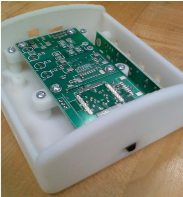
Fig. 13.14. Manufactured Enclosure with MAIN PCB and ONE BANK OF LEDS INSERTED.
