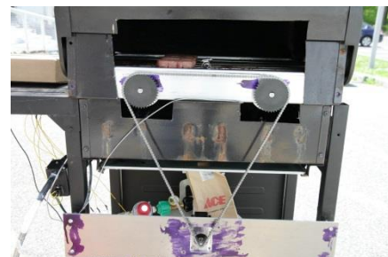
Fig. 15.12. Chain Drive for Flipping Mechanism.
