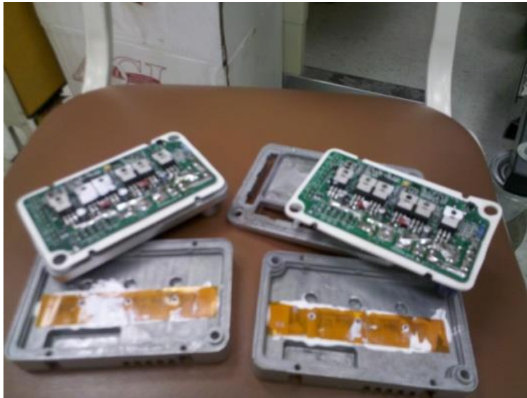
Fig. 11.3. The Failed Brushless Motor Drivers.
