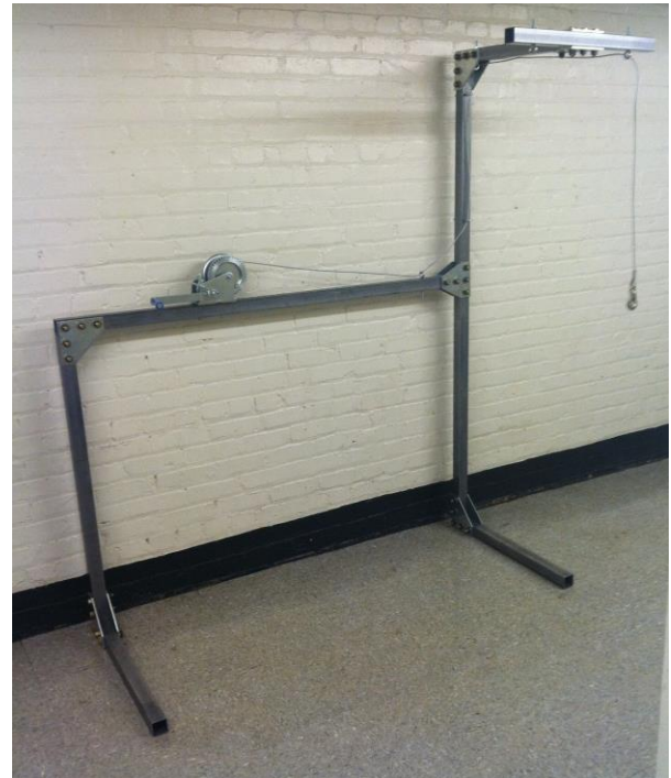
Fig. 19.3 Photo of the One Leg Up Device before it was powder coated in white and attached to her bed. The left side of the frame is toward the head of the bed, where the client can reach the winch, and the clients legs are attached to the part of the frame that cantilevers over the bed. The legs at the bottom of the frame will attach to the bed.
