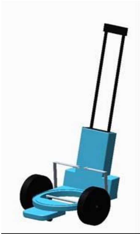
Fig. 16.4. Bumbo Baby Seat Wheelchair Trainer: (Left) CAD drawing; (Right) Child at Hand-in-Hand using the device [picture released with parental consent].
