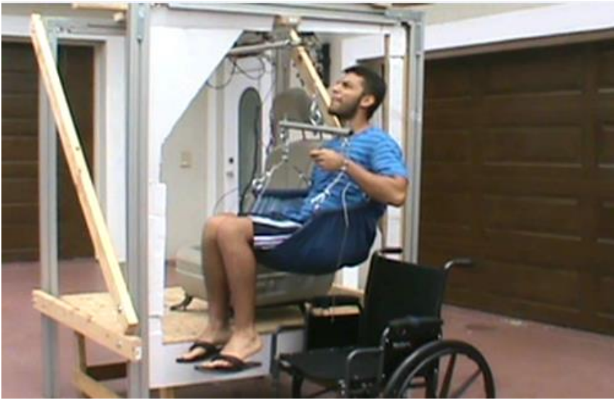
Fig. 8.17: Rail Lift Mechanism.
